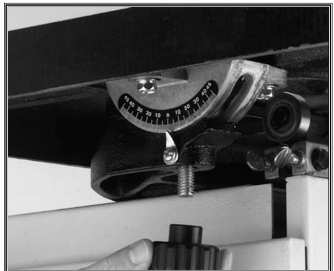
Figure 18. Securing table with the hand knobs.
